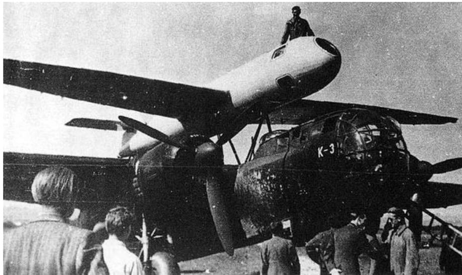
sitting in the conventional fashion made the pressure vessel too big so the pilot was given a couch and would fly the aircraft from the prone position, making pressurisation much simpler. In case of emergency the pressurised cabin could be jettisoned from the rest of the aircraft so the pilot inside it could fall to a safer altitude before parachuting to safety.
