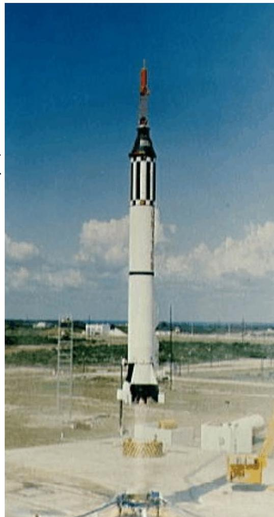
were extended by 96 inches to increase their fuel capacity and give them an addition 20 seconds of burn time. They were also fitted with more advanced A-7 motors and given about 800 engineering changes to qualify them as a manned space launch vehicle.
