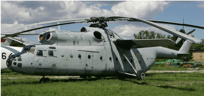
payload greater than the total weight of the West's largest helicopter, the Sikorsky S-64A. To reduce stress on the engines, transmission system and rotor blades the Mi-6 could also be fitted with stub wings for ferry and long range flights which took about 20 percent of the load and allowed it to fly at up to
